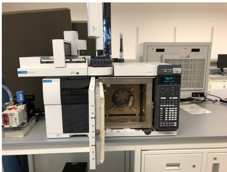
A GC in EEEL with the oven door open to show the coiled column within
