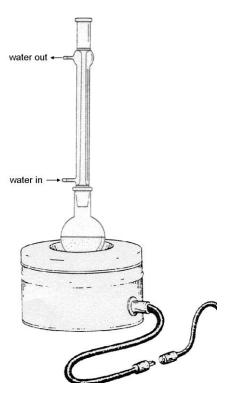
**NOTE**: In the equipment set up shown here, a heating mantle with a heating controller is being used to heat the round bottom flask. In your equipment set up, the heating mantle and heating controller will be replaced by an engineered (shaped) aluminium block sitting on the top of a stirrer hot plate. This is a more modern version of a heating mantle with some distinct benefits.
