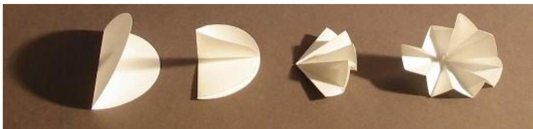
The steps to flute the filter paper are shown. First, fold in half; open and fold in half at 90° to the first fold, subsequently align adjacent folds and make new folds bisecting the previous folds until a fan-like arrangement is obtained. Pleat into a fan by folding each segment in the opposite direction to its neighbours, in accordion-like fashion. When opened out the complete fan-like fluted paper results.
